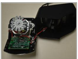
• Using the Phillips #2 screwdriver, remove these six screws (13mm long, 6mm head diameter). Then carefully remove this layer, and rest it next to the blender base.
