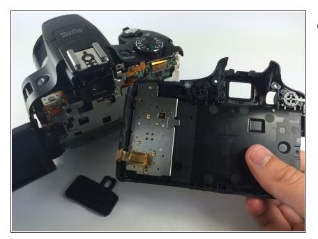
Now you can completely separate the back encasement from the rest of the camera.
