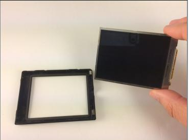
Use your fingers to remove the LCD screen from its encasing. It comes out very easily.
