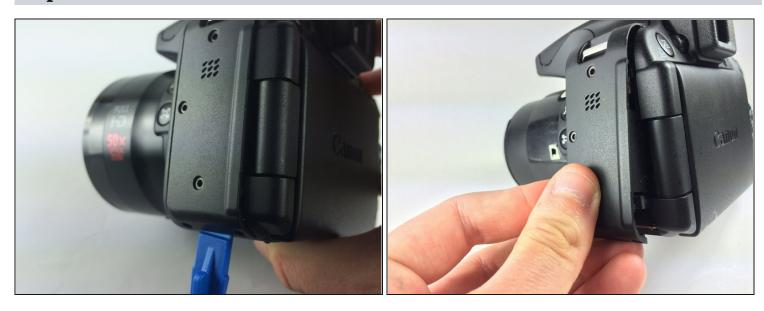
• Use the plastic opening tool to carefully start lifting up the camera's left-side panel. Then use your fingers to pry off the rest.
