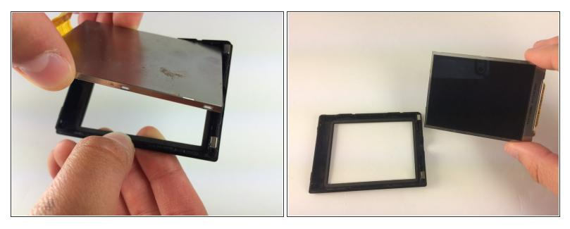
• Use your fingers to remove the LCD screen from its encasing. It comes out very easily.
