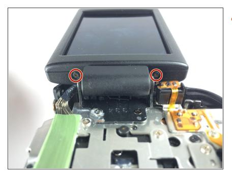
Remove the Phillips #000 screws, length 3 mm, on the inside edge of the LCD screen panel.
