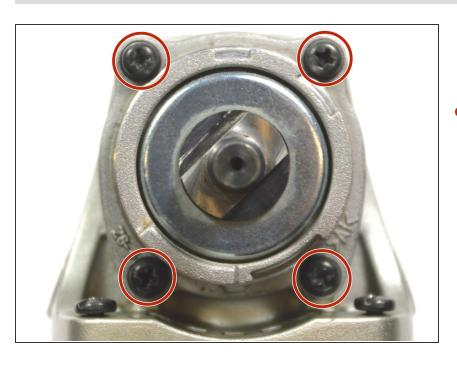
Unscrew the four 15 mm pan head screws using a Phillips #02 screwdriver.
