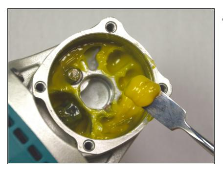
Use a metal spudger to scrape the old grease from the cavity.
