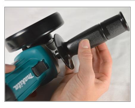
Unscrew the handle unit until it is removed completely.
