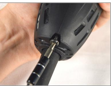
Unscrew the 20 mm tapping screw using a Philips #02 screwdriver.
