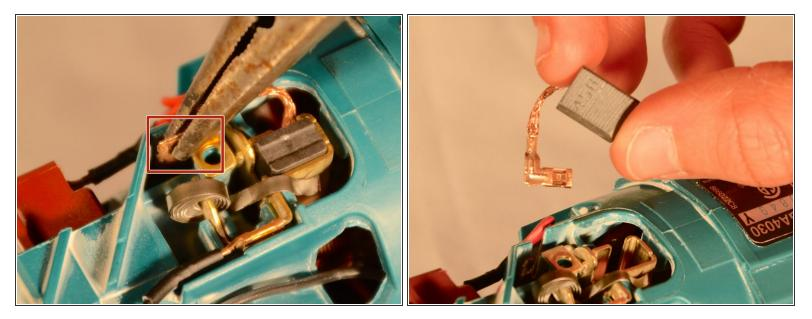
• Use needle nose pliers to gently pull out the carbon brushes by their crimped connectors.
