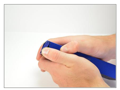
Slide out the rubber foot located on the bottom of the case.
