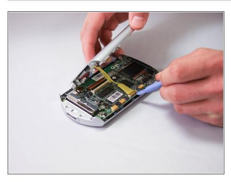
Using the plastic opening tool, carefully detach the yellow ribbon from the connector pins to separate the device into two halves.
