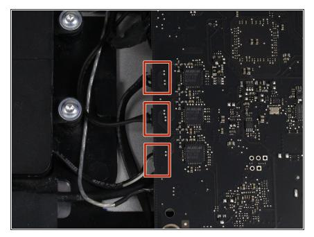
To the right of the middle speaker is the logic board. Here is where the three speakers in the display are connected and need to be removed.
