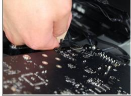
• For the first of the four wires (furthest away from the wire that is held in by a screw), grab onto the connector and pull slowly.
