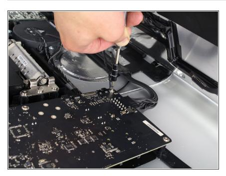
For the last wire connecting to the LCD, use your T 10 Screwdriver to remove the screw.
