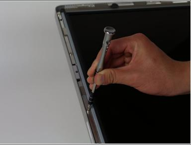
Unscrew the 12 screws around the side edges and the top of the LCD with the TR 10 Screwdriver.
