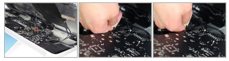
For the first of the four wires (furthest away from the wire that is held in by a screw), grab onto the connector and pull slowly.
