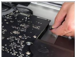
For the connector on the other side of the logic board, grab the connector from underneath and carefully pull it from the board.
