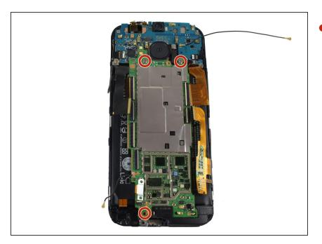
Remove three silver 3mm screws using T5 screwdriver.
