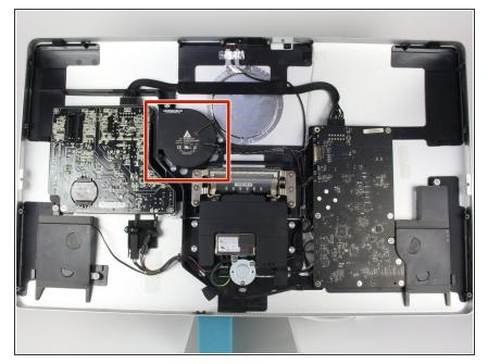
Now you should have access to the rest of the display. From here, locate the fan.
