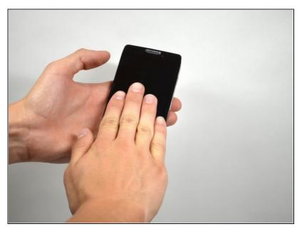
Holding the device in your hand, push the screen towards the top of the phone until it disconnects from the base of the phone.
