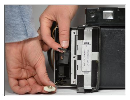
Carefully remove the battery from the positive and negative terminals.
