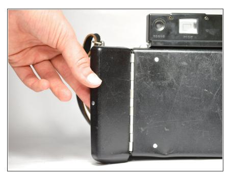
Open the battery compartment on the back left of your Polaroid.
