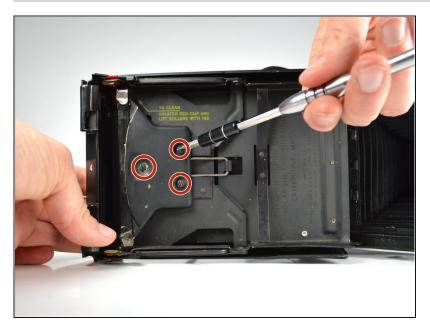
Unscrew the three 2.5 mm screws (attached to the metal plate) with a 3.0 flathead screwdriver. Then take off the metal plate.
