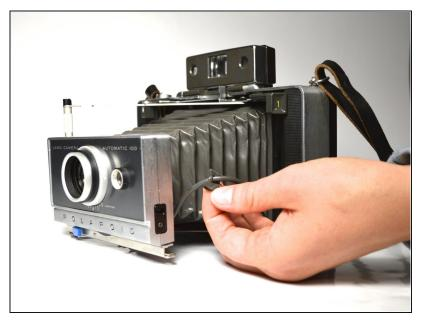
• Peel the two battery cable tabs off of the bellows.
