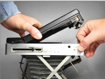
• Open the back cover by pushing the lever on the bottom towards the left.
