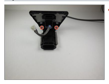
The subwoofer air tunnel can be removed by unscrewing the 2 XXXX screws with a Phillips #2 screwdriver.
