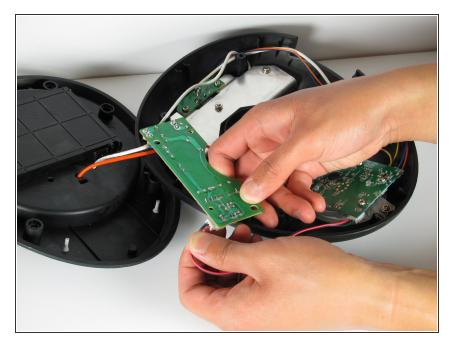
• Lift the motherboard out of the device
