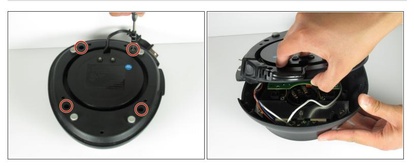
Remove the four 12 mm Phillips #2 screws surrounding the base then lift the bottom half of the base to expose the circuit boards inside the device.
