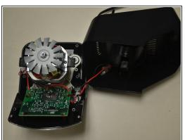
Using the Phillips #2 screwdriver, remove these six screws (13mm long, 6mm head diameter).
