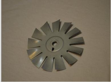
Slide the washer and fan off of the screw.
