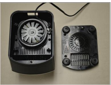
Remove the five screws (13mm long, 6mm head diameter) using a Phillips #2 screwdriver.
