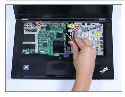
• Remove the three 5mm screws holding the palm rest casing in place using the Phillips #0.
