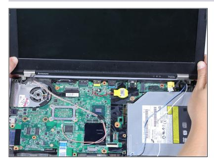
• Remove the LCD screen unit by holding the sides and lifting it upwards.
