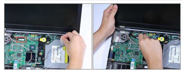
• Unplug the two black cables that connect the screen to the motherboard.
