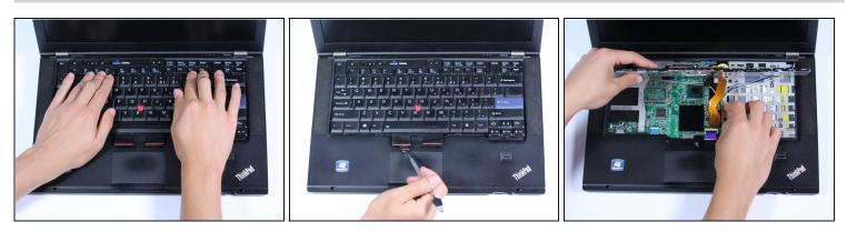
• Gently push down on the keyboard and slide it towards the screen. This will pop the bottom of the keyboard out of the casing.
