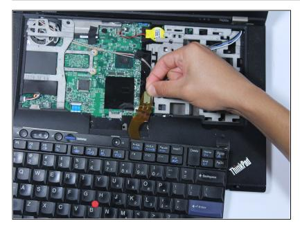
• Remove the orange cable by lifting up on the tab on the end of the ribbon connection.
