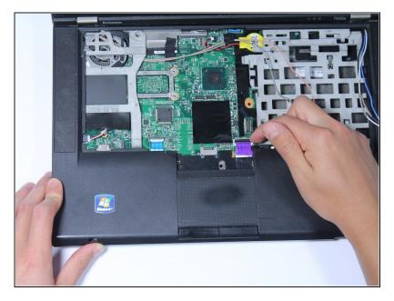
• Lift up the black retaining flap holding the purple ribbon cable in place, and carefully slide out the ribbon.
