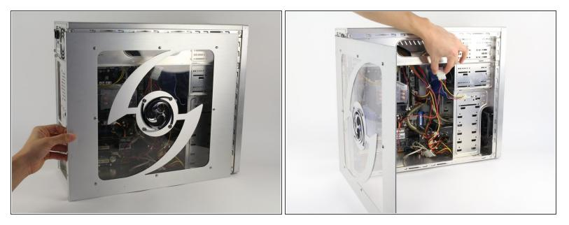
• Next, remove the side panel of the computer case to allow access into the computer. Slide the panel towards the back of the computer and lift it up to remove.
