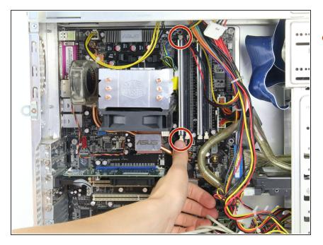
Unlock the RAM by pressing down on the tabs from either side of the RAM that are securing the RAM to the socket.
