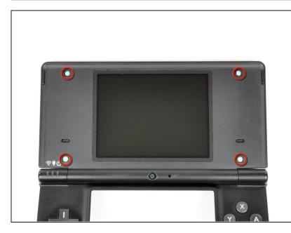
• Remove the four Phillips screws securing the rear bezel to the front bezel.
