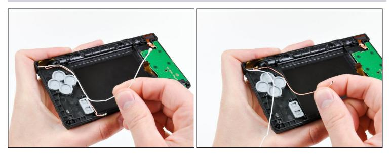
• De-route the microphone and Wi-Fi antenna cables through the opening located on the bottom DSi's framework.
