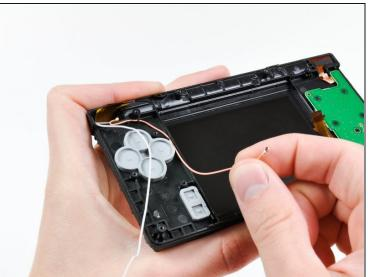
De-route the microphone and Wi-Fi antenna cables through the opening located on the bottom DSi's framework.
