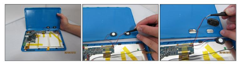
now that the case is open, carefully remove the speakers and set aside.
