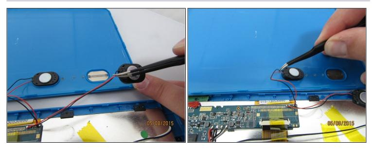
• Gently remove the speakers from the back case with tweezers and set the case aside.
