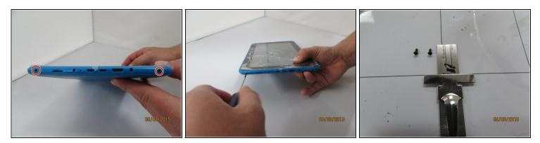
Remove the 3mm screws from bottom of tablet with the precision screwdriver and place on <u>magnetic mat</u>. label where they came from.
