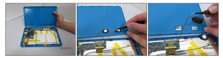
• now that the case is open, carefully remove the speakers and set aside.
