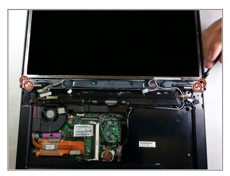
Using the T9 Torx screwdriver, unscrew the four 4mm screws.
