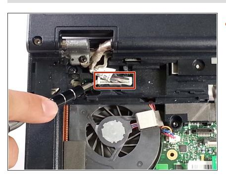
Using a flathead screwdriver, work both sides of the connector next to the fan and take it out.
