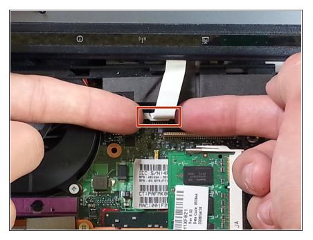
Put a finger under each side of the plastic lock on the ribbon cable and pull up.
