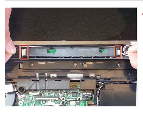
Using your fingers, take out the two connections near the hinges.
