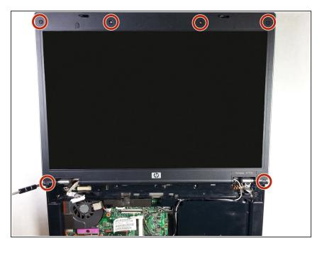
Using the blue plastic opening tool, pull the rubber covers off the screen screws.
