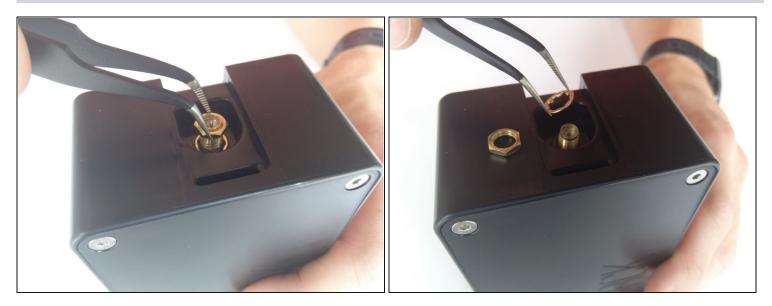
• Remove the nut and washer from the RF connector, located where the antenna was connected.
