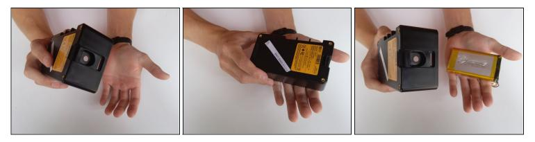
• Flip device upside down. Hold the device and tap into your other hand with varying force to remove battery.
