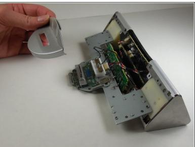
Remove the plastic dock cover by using two fingers to push the attached metal piece forward and slide it out of the holes.
