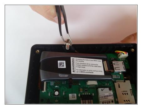
Remove the connection located on the edge of the modem.
