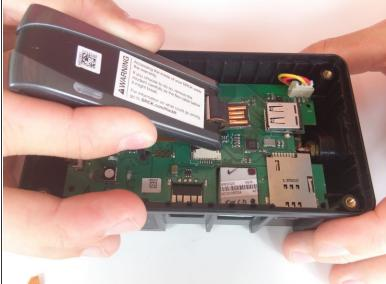
Remove the modem from the device.
