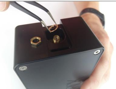
Remove the nut and washer from the RF connector, located where the antenna was connected.
