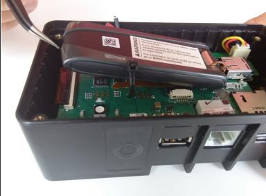
Slightly lift the modem to reveal the brown ribbon connector and metal connection plate, located on the bottom of the modem.
