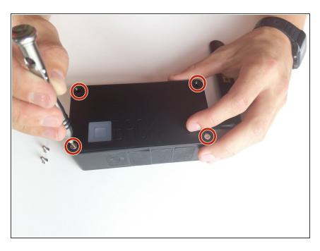
Remove the four screws(4mm hex head) on the corners of the device with a Hex 2.0 Screwdriver.
