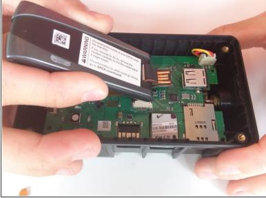
Remove the modem from the device.
