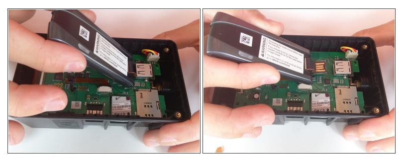
• Remove the modem from the device.
