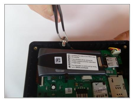
• Remove the connection located on the edge of the modem.
