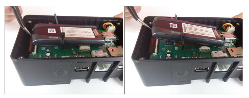
Slightly lift the modem to reveal the brown ribbon connector and metal connection plate, located on the bottom of the modem.
