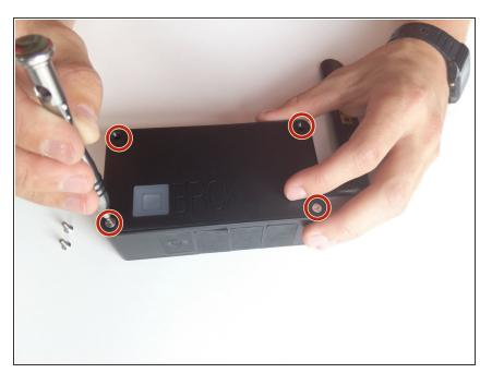
Remove the four screws(4mm hex head) on the corners of the device with a Hex 2.0 Screwdriver.
