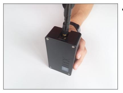
Stand the device on its side so the antenna is sitting on the top.
