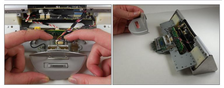
• Remove the plastic dock cover by using two fingers to push the attached metal piece forward and slide it out of the holes.
