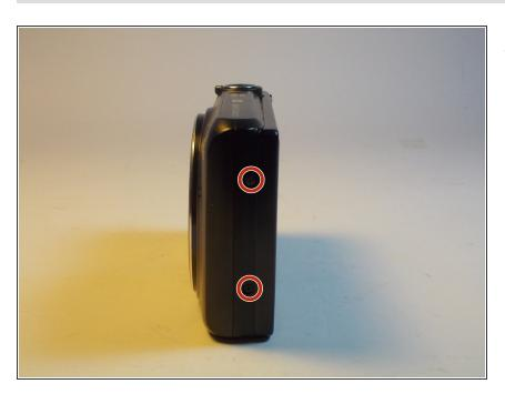
Rotate the camera to the left side and remove the two, black, #00 Philips screws.
