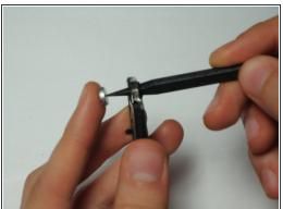
With the LCD unit removed, gently press out the speaker with a non-metallic pointed object.
