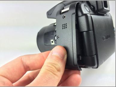
Use the plastic opening tool to carefully start lifting up the camera's left-side panel. Then use your fingers to pry off the rest.
