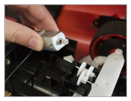
Remove motor. Lift the servos core motor out of the motor housing. Be careful not to pull out the plastic gears while doing so.
