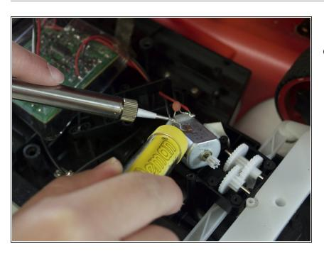
Solder wires back on. The last step will be to solder the red wire back on the left side of the motor and the black wire back on the right side. You can do this by referring to this how to solder/desolder page. To reassemble your device, follow these instructions in reverse order.
