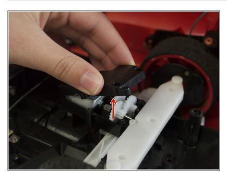
Remove top cover. Lift the panel off the top of the motor and place it back with the wires.
