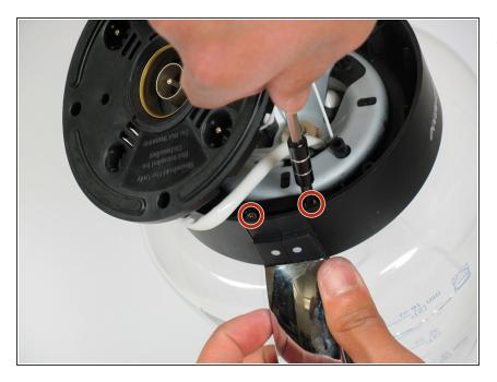
Locate the two 10 mm Phillips #2 screws at the bottom of the handle and remove them.
