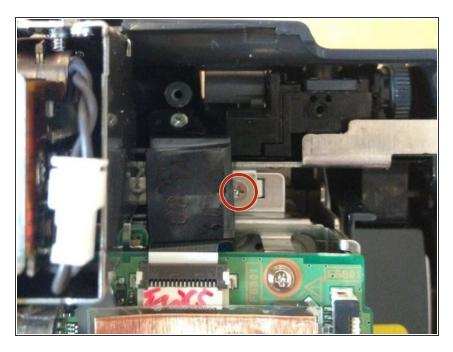
Remove the 3mm screw using the metal spudger.
