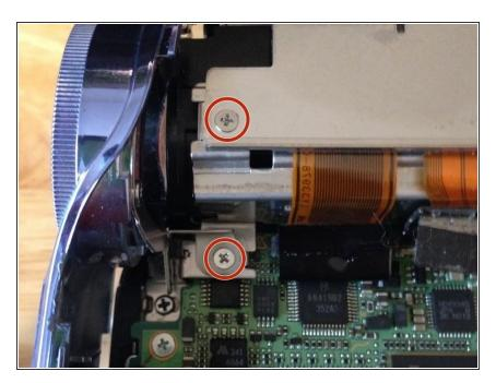
Remove the two 3mm screws using the PH0 screwdriver.
