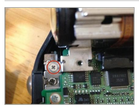
Remove the blue dust cover using the metal spudger. Unscrew the 3mm screw using the PH0 screwdriver.
