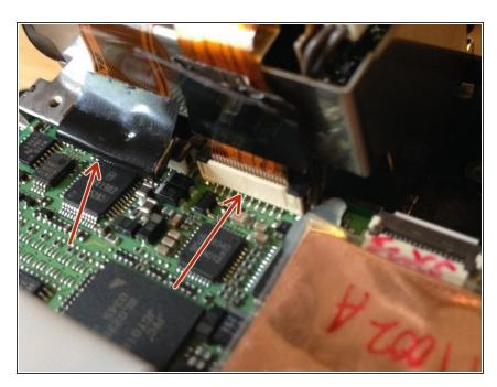
Remove the two logic strips by lifting the plastic clips using the metal spudger.
