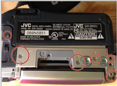
Unscrew two 3mm Phillips #0 screws. Then remove 6 3mm Phillips #0 screws from the bottom of the camera.
