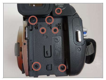
Unscrew 3mm Phillips #0 screws from the batter port under the eye piece.
