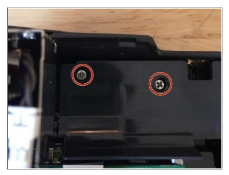
Remove the two 5mm screws using the PH0 screw driver. Use the metal spudger to remove plastic casing.
