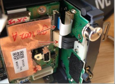
Now the camera can be split into two pieces. Be careful when removing the two sides and remove
