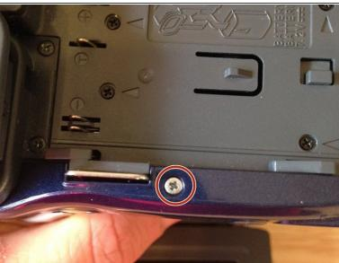
Unscrew two 3mm Phillips #0 screw from the bottom of the camera to remove blue plastic casing.
