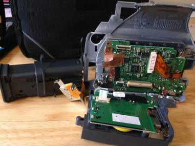
Unscrew 3mm Phillips #0 screw and disconnect cable. This will disconnect the eye piece from the camera.
