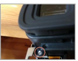
• Unscrew two 3mm Phillips #0 screws from around the eye piece. Then flip the camera over and unscrew 3mm Phillips #0 screw. Then unscrew 3mm Phillips #0 screw from under the eye piece.
