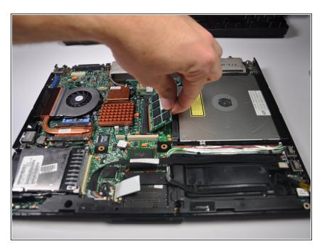
Remove the chip by lifting up the side closest to the cd drive first.
