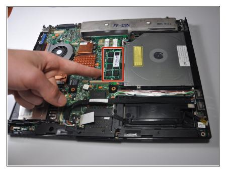
Recommended: First, remove the second RAM chip, in the center of the motherboard. The chip is rectangular, with black squares and a "transcend" label on it.
