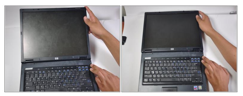
Open up the laptop so that the screen is facing towards you. Push the monitor back until it is flat, parallel to the keyboard.
