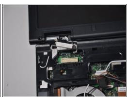
• Unplug the black cable with rectangular white plastic head from the motherboard. It is located at the top left of the motherboard, directly below the left hinge.
