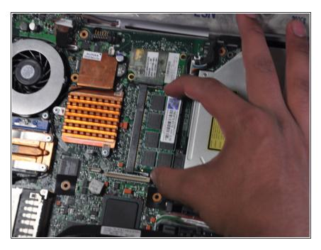
To remove the chip, locate the two metal clips on the top and bottom of the chip. Clamp them in towards the RAM chip and hold.
