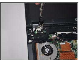
Remove the two 9.8mm 3.0 flathead screws. There is one at each of the hinges.
