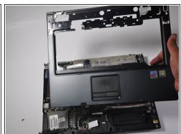
Unplug the white cord connecting the mousepad to the motherboard from the motherboard, and pull off the entire plastic panel.
