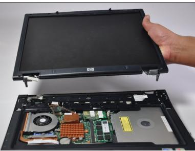
• Pull the monitor directly upwards from where it lay. The two metal hinges should easily slide out of their holes and the monitor will be disconnected from the motherboard.
