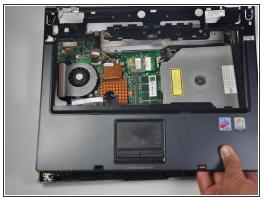
Using the iFixit opening tool, pry the black plastic panel (with mousepad) off of the motherboard.
