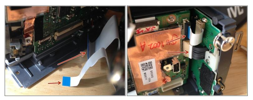
Now the camera can be split into two pieces. Be careful when removing the two sides and remove the cables connecting the two halves. There are also cables that need to be disconnected from the battery pack section.
