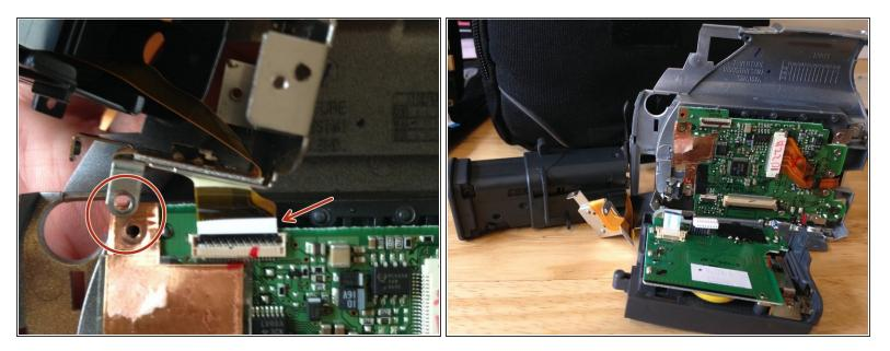
Unscrew 3mm Phillips #0 screw and disconnect cable. This will disconnect the eye piece from the camera.
