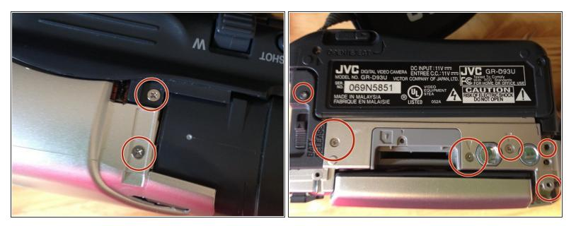
Unscrew two 3mm Phillips #0 screws. Then remove 6 3mm Philips #0 screws from the bottom of the camera.
