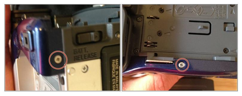
• Unscrew two 3mm Phillips #0 screw from the bottom of the camera to remove blue plastic casing.
