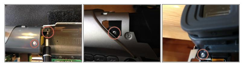
Unscrew two 3mm Phillips #0 screws from around the eye piece. Then flip the camera over and unscrew 3mm Phillips #0 screw. Then unscrew 3mm Phillips #0 screw from under the eye piece.
