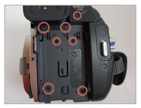
Unscrew 3mm Phillips #0 screws from the batter port under the eye piece.
