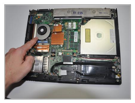
Locate cooling fan directly to the left of copper heat sink.
