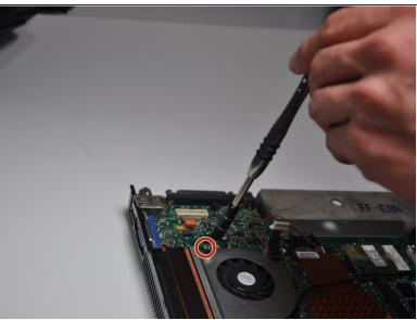
Locate and remove the two 7.0mm Phillips #1 screws on the top left and top right corners of the cooling fan.
