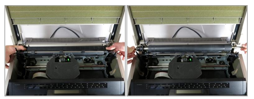
• While both spring levers are depressed, lift up with both hands to remove the roller wheel.
