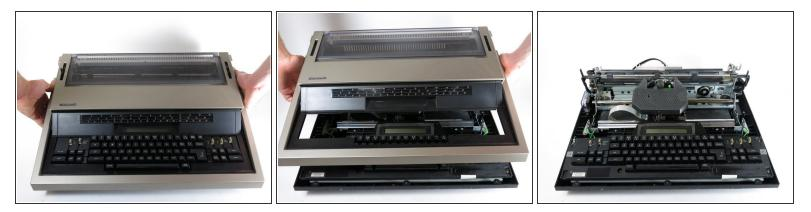
• Flip the top down. Then, with both hands, lift straight up on the tan case to remove it from the chassis.
