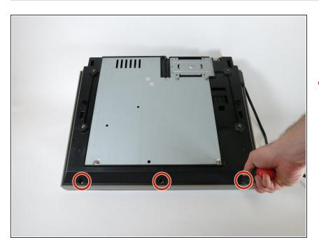
Remove the three 19 mm screws located in the recessed holes on the edge of the black underside panel using a Phillips #2 screwdriver.
