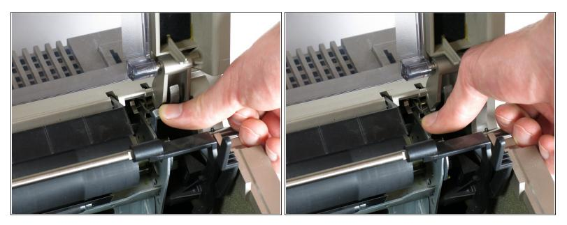
• Unlock the roller wheel by simultaneously pressing down on the two spring levers on the left and right of the roller ends.
