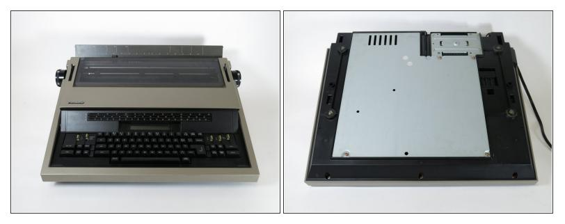
• Flip the typewriter to expose the bottom body panel.
