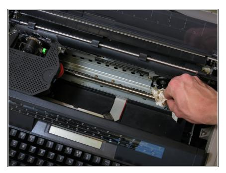
Wipe down the rails with a clean cloth to remove any debris, making sure to clean around the carriage.
