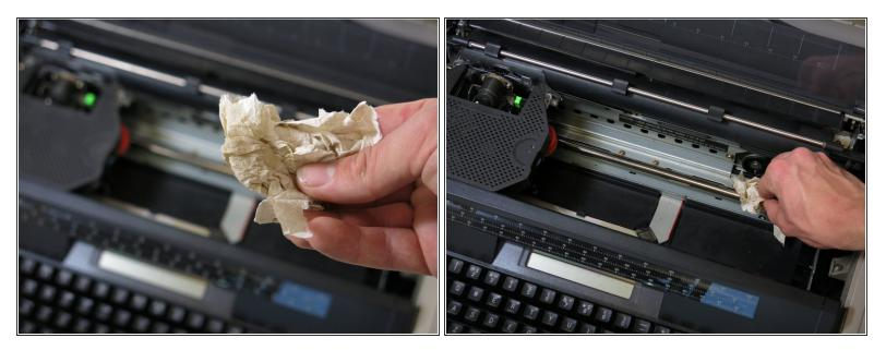
Place several drops of the oil-based lubricant onto another clean rag, and wipe down the rails.
