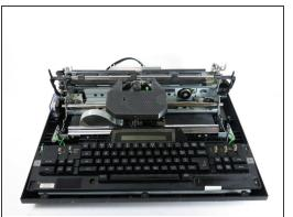
Flip the top down. Then, with both hands, lift straight up on the tan case to remove it from the chassis.
