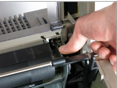
Unlock the roller wheel by simultaneously pressing down on the two spring levers on the left and right of the roller ends.
