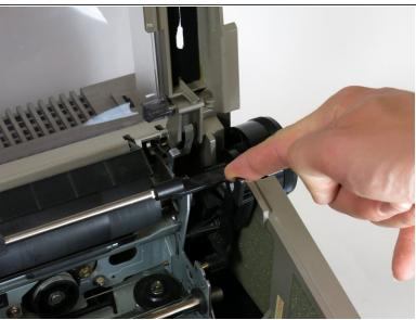
Flip the plastic lever on the right side of the roller wheel to disengage the paper lock.
