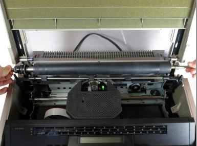
While both spring levers are depressed, lift up with both hands to remove the roller wheel.
