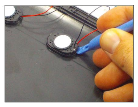
• Use a plastic opening tool to pry the speakers out of the rear case.
