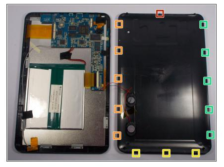
The clips will be released in the order specified as the spudger tool is moved along the seam around the device.
