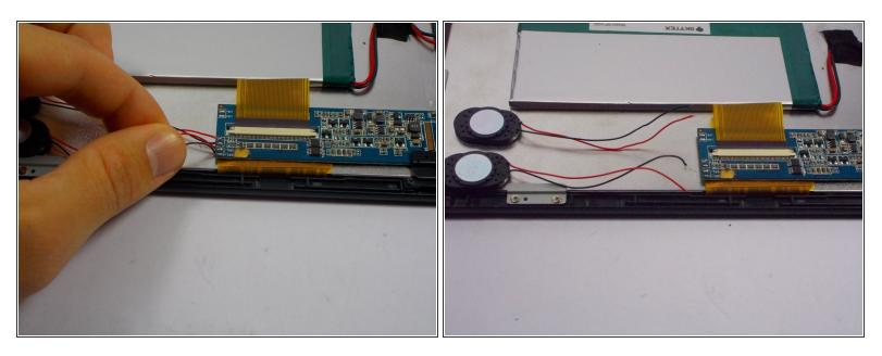
• Use a soldering iron and desoldering braid to desolder the two sets of red and black wires.
