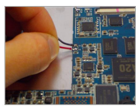
Use a soldering iron and desoldering braid to desolder the red and black motherboard battery connections.
