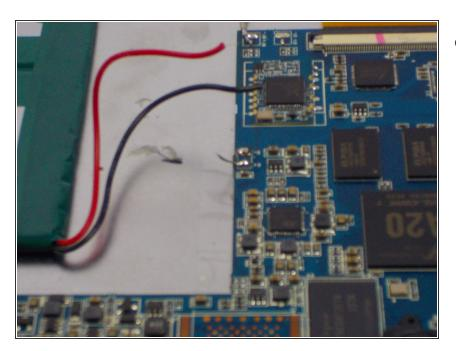
Gently lift the battery up and out of the device.
