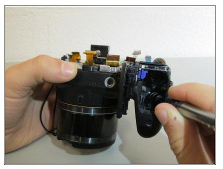
On the top of the inside the battery compartment, remove the #00 6.0 mm Phillips screw.
