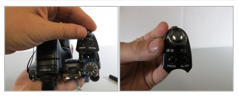
• Lift the button housing from its position on top of the camera.
