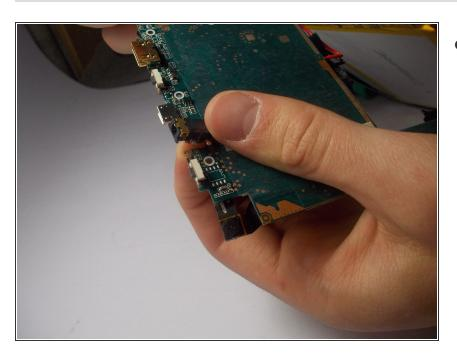
Pop the audio jack out by applying pressure on the side that is flush with the front of the circuit board.
