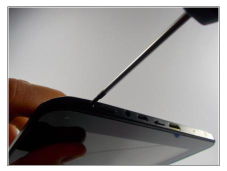
Begin by unscrewing the two 1.4 mm diameter Phillips #00 head screws at the top of the device.
