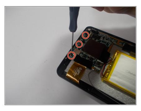
Remove the three 1.4 mm diameter screws anchoring the circuit board in place with a Phillips #00 head screw driver.
