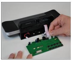
• Disconnect the four cables connecting the motherboard to the device.
