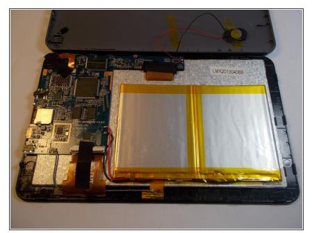
Remove the soldering of the wires coming from the battery connected to main circuit board. Also, remove the tape.
