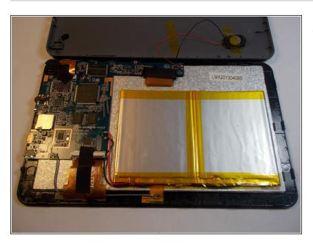
Replace the old battery with a new one and solder the wires of the new battery as shown on the main circuit board.
