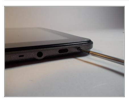
Unscrew and remove the screws from the top of the tablet.
