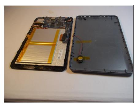
Remove the back cover of the tablet.
